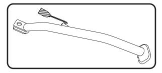
3. Install (No. 12/13) 11660-BRKT-L/R, left and right muffler hanger brackets where passenger footpegs where removed using (No. 5) M8X20, bolts and (No. 7) 8MMNUT, nuts. See diagram for proper orientation and order of hardware. Do not torque at this time.
